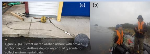
Figure 7: (a) Current meter washed ashore with broken anchor line. (b) Authors deploy water quality sonde to collect environmental data.
